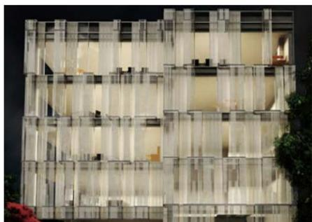
The shroud expresses a vertical aesthetic, which is emphasized by a floor-to-floor glazing, 3 meters tall. The expression is further reinforced a varying scales from the exterior channel glass baffles to the custom vertical frit pattern to interior vertical window treatments, all together creating a richness in its depth.
