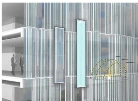
The primary façade comprises of high performance DGU with low-e coating with roughly 50% of glazing with custom frit pattern. The DGU (supplied by Saint Gobain) is composed
